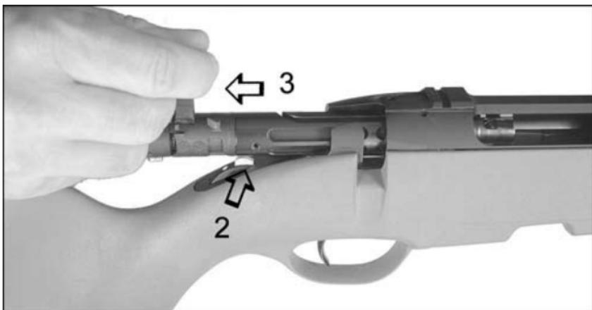
3. Hold bolt by the bolt handle and extract it from the receiver.
