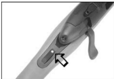
Turn bolt handle 70° upwards to unlock the bolt. Pull bolt all the way to the back by the bolt handle.
