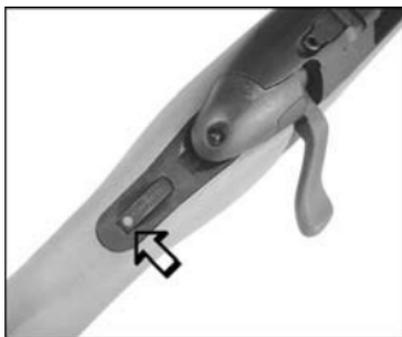
By retracting the bolt, the spent cartridge shell will be extracted and ejected. Moving the bolt forward will feed a new cartridge into the cartridge chamber of the barrel. Relock the bolt by turning the bolt handle. Move rotary safety back to position **“Safe”**. The rifle is loaded, cocked, and safe, again. If the safety has been released, but no shot fired, the weapon must be immediately put on safe again.
