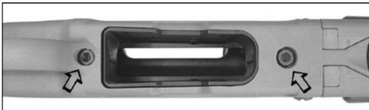
Turn in screws (1) of HC-KIT and tighten it with a torque wrench (9 Nm). It is recommended to secure the screws with glue Loctite 242.
